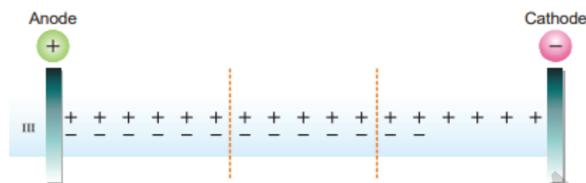
Figure 25.5 With silver electrodes, concentration around the cathode falls while it increases around the anode.
